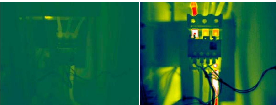
Figures 2a and 2b - The left image shows an IR image that is not properly thermally tuned. The much clearer image on the right is correctly thermally tuned.
